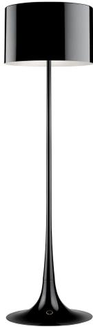
Floor fixture providing diffused lighting. Spun metal frame and diffuser, die-cast aluminum diffuser support arms and lamp-holder support, painted in the colors indicated below. White, injection-molded polycarbonate diffuser supports. On the cable there is the electronic dimmer which allows the regulation of light brightness.
